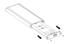
Step 2: The SSD corresponding to the seat and PCBA connection good, then lock it. Pass into the aluminum and the SSD after locking the back cover.
